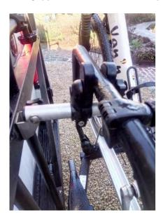
You can also remove the clamp from the tube and turn it around with the star knob pointing to the inside.
