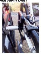
When you tighten, you can choose to position the frame holder higher or lower by turning the mounting bracket half a turn.
