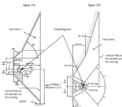
To obtain this clear space when towing a trailer in combination with an installed Van 'n Bike bike carrier rack, one can temporarily remove the ball coupling on the Van 'n Bike bike carrier rack, or an extended tow hook on the tow bar on your vehicle can be a solution. The user must immediately contact the manufacturer for an explanation of the instructions.
