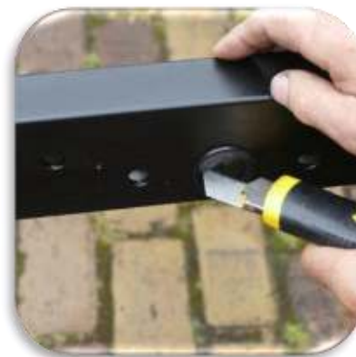
Tighten the spacer bolts onto these attached screws (2 per lamp)
