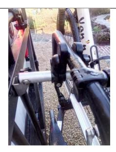
You can also remove the clamp from the tube and turn it around with the star knob pointing to the inside.
